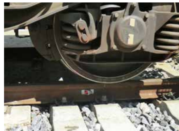
RSMP15 for surveying with robotic total station while under load.
