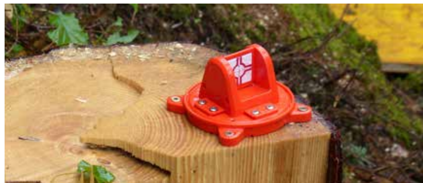
Example of the use of RS193rM as a fixed point on different surfaces and for the exact alignment of the drill carriage.
