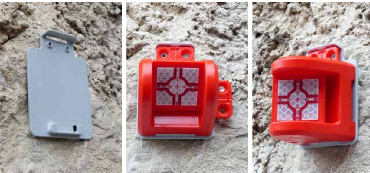
RS183 on mounting plate RSFP-X80g for simple and fast mounting on any base. Simply click out, turn and click in again to survey in both horizontal and vertical orientations with the same survey point.
