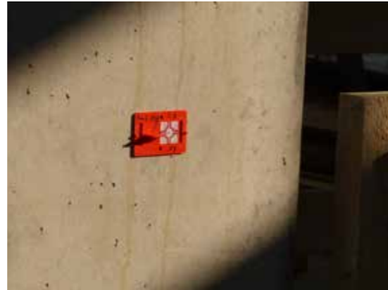
RS30r in industrial construction: a perfect measuring point for each measuring instrument.
