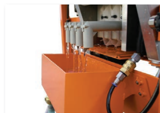
Filter outlet with drain gutter
