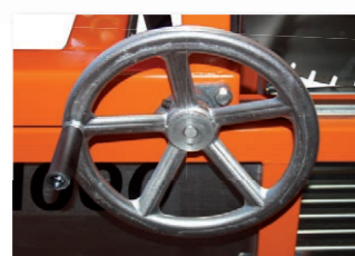
moving of the cutting head by hand wheel
