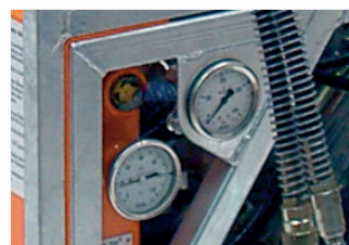
Oil temperature and pressure controls
