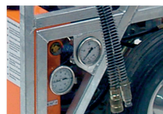
Fully galvanized frame
