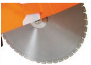
Max blade size 800 mm (cutting depth 310 mm)
