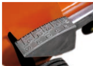
Cutting depth indicator
