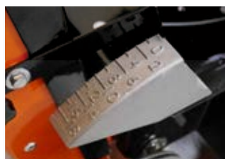
Cutting depth indicator
