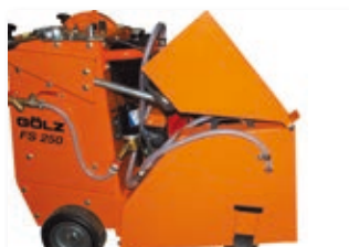
Divisible blade guard - can be raised for intersections
