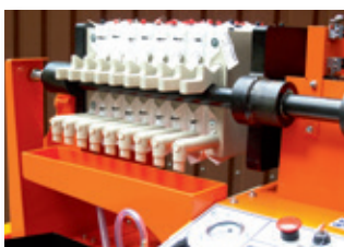
Filter cakes fall into collection container
