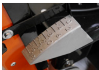
Cutting depth indicator
