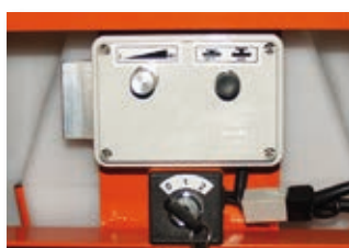
electric start - control panel for adjustable speed
