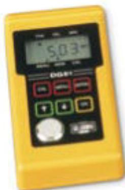
DG 51 B has been developed for standard measurement as well as for application when gain adjustment is necessary according to surface condition and/or the state of corrosion. The V-path automatic correction provided for carbon steel, stainless steel and aluminium, allows maximum accuracy. Correct coupling and underthickness display indications are provided as well as display freezing of minimum value detected.
